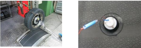
FIGURE 4: Tire test rig (left) with embedded prototype (right)
