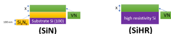
FIGURE 2 : TYPES OF SUBSTRATES USED, (SiN) USED FOR ELECTROCHEMICAL TESTING AND (SiHR) FOR RESISTIVITY (CONDUCTIVITY) TESTING
